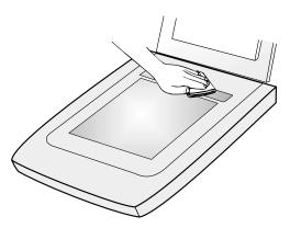
3 Clean the glass using a soft, lint-free cloth sprayed with a mild glass cleaner.
